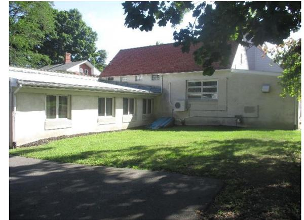
Rain gardens adjacent to the buildings can capture, treat, and infiltrate roof runoff. Existing downspouts on the western building can be disconnected and rerouted to the rain garden. The downspout on the eastern building is already disconnected. A preliminary soil assessment suggests that the soils have suitable drainage characteristics for green infrastructure.
